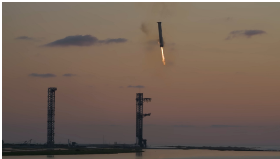
(a) "Booster 12" approaches the tower with three engines running for the final descent
