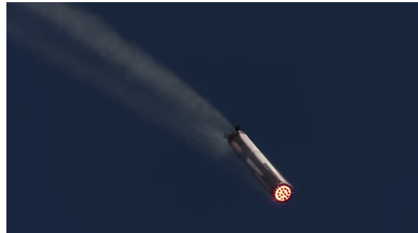
(b) The Super Heavy endures air friction at 4000\text{km}/\text{h} , notice the very visible angle of attack
