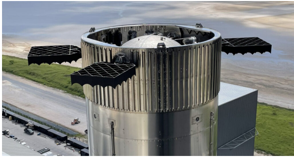
(a) Super Heavy and its grid fins. They have rotation around their axis as their only degree of freedom.
