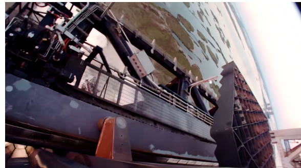
(b) The Super Heavy landing pins making contact with the arms' rails
